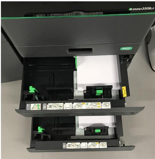
Adjusting the MFP's paper drawers for different-sized media is very easy; users simply press the locking clips in and slide to the required size. In addition, paper limit indicators are easy to see which reduces the risk of users overloading the drawers.
