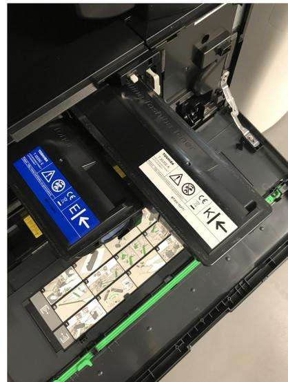
Replacing black and erasable blue toner on the MFP is simple and clean, but toner cannot be replaced on the fly.
