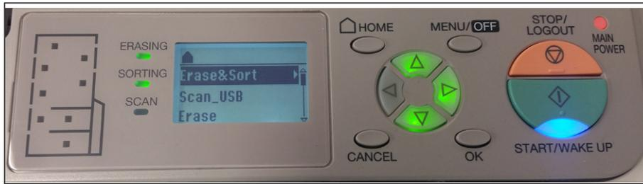
The RD301's control panel has a four-line LCD display, a device graphic with LED lights to indicate where misfeeds are located and various hard key buttons for users to use to navigate the menu options. At an administration level, the control panel is more limited than that of the MFP, plus entering information involves multiple key presses which is time-consuming; most functionality is easily managed in the web utility.
