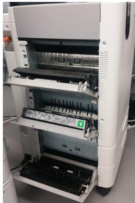
Reusable and rejected paper is neatly sorted into separate paper drawers for easy identification; misfeed areas (right) are easy to access.
